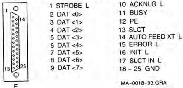
Figure B-3 Parallel Printer Port (Bidirectional)
